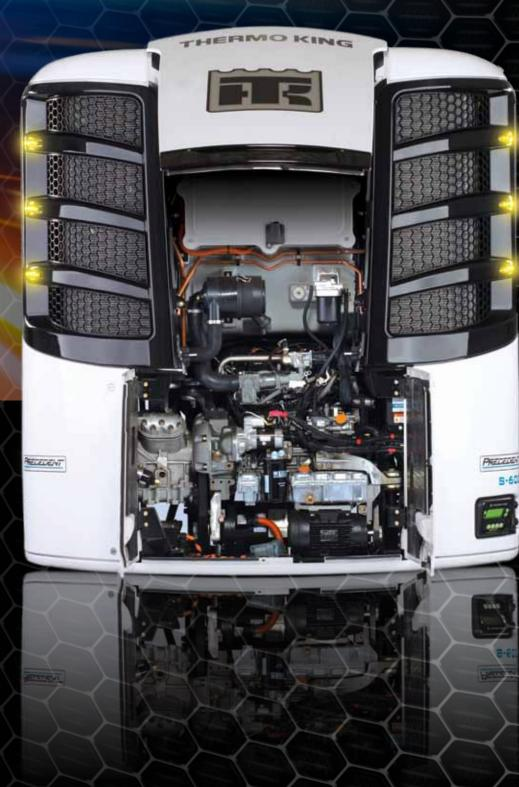
S-Series models, which include the S-600 and S-600M, already meet Tier 4 final emissions certification by the Environmental Protection Agency (EPA) and California Air Resources Board (CARB). Further, they comply with CARB's Ultra-Low-Emission Transport Refrigeration Unit In-Use Performance Standards (ULETRU).
